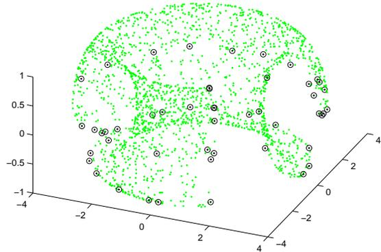
Figure 21: Boundary detection of incomplete tire
