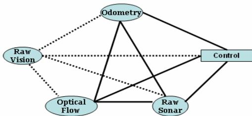
**Figure 4 – Undirected graph for the host of sensors and motor output used for the experiments. The solid lines represent stable mappings as determined during training, while the dotted lines represent mappings that have been ruled out during training.**
