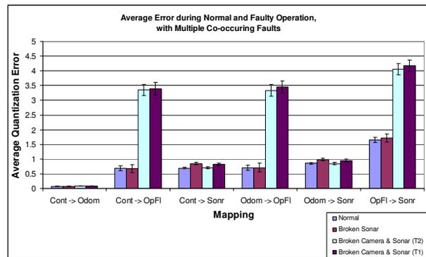
**Figure 8 - Average quantization error with multiple co-occurring faults, for each mapping. T1 indicates training with normal data, and T2 indicates training with only faulty data.**
