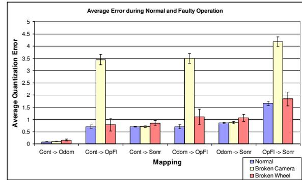
**Figure 6 - Average quantization error with wheel and camera faults, for each mapping.**
