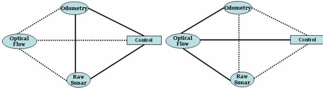
**Figure 5 – Mappings during camera (left) and wheel (right) faults. Solid lines indicate mappings that have remained stable despite the faults, and dotted lines indicate mappings that have not.**
