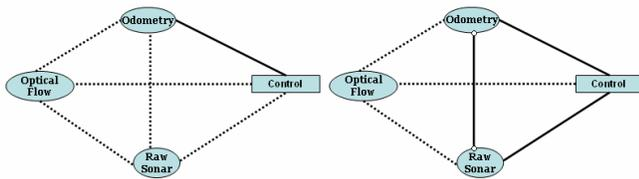
**Figure 7 - Mappings with multiple co-occurring faults (both camera and sonar faults). Left: Mappings after training on normal data. Right: Mappings after training after only the sonar fault, hence isolating the camera fault.**
