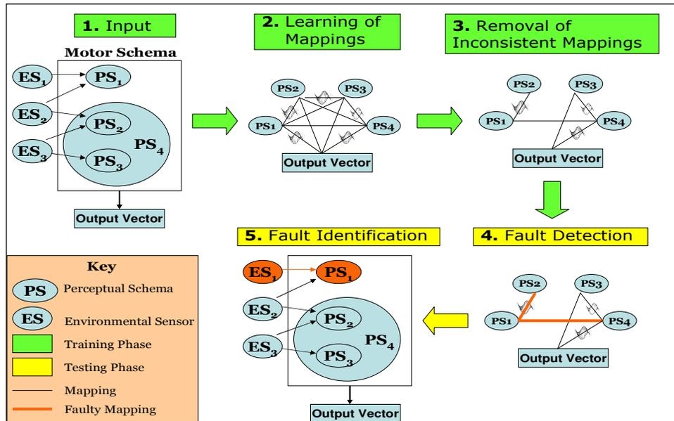
**Figure 2 – Steps involved in the detection and identification of changes in the perceptual and motor capabilities of a robot in our system.**
